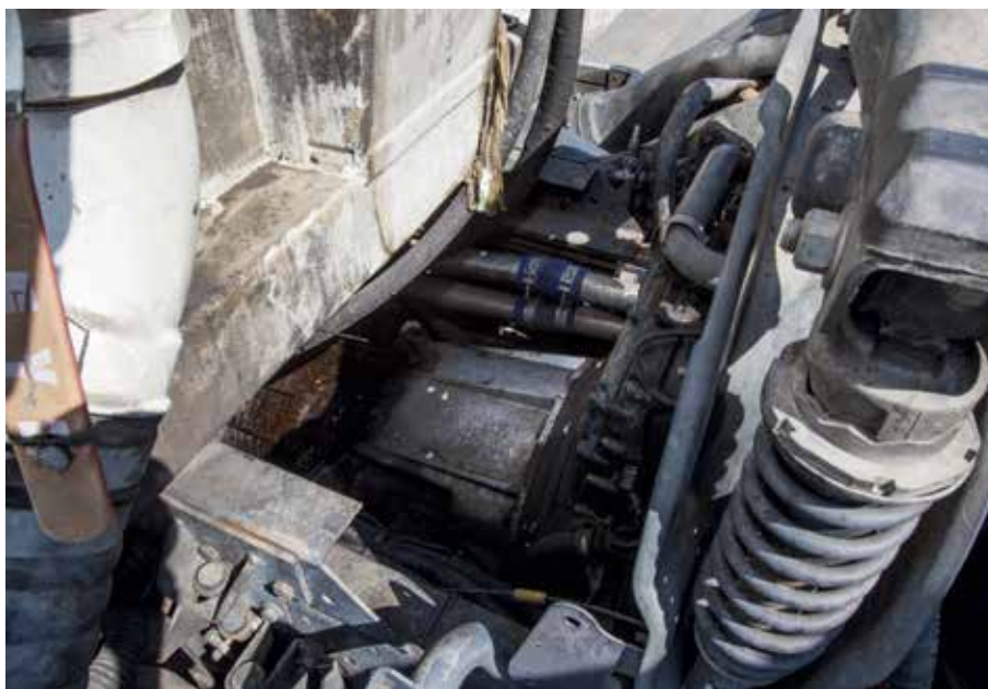
The gearbox cooling system was designed and executed at Driveline's facilities
