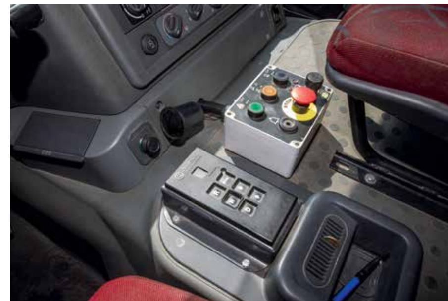
The position of the new gearbox selector was looked into, in order to bring about ergonomics of use
